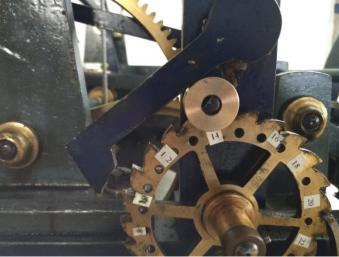
STRIKE – push the silencing bar to the right and insert the spacer as shown. Re-activate by removing the spacer.
